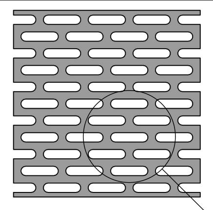
Slot Size: LR1(5) X LR2(25) Staggered Length: Z1(30) X Z2(16)
